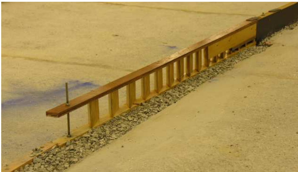
Figure 9: Layout C, upstream: final layout of the openings, seen on the scale model.
