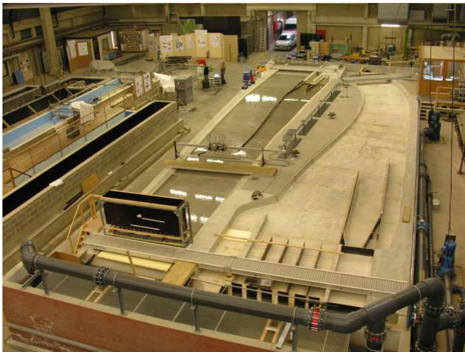
Figure 3: Physical model of the new lock of Ivovz-Ramet approaches.
