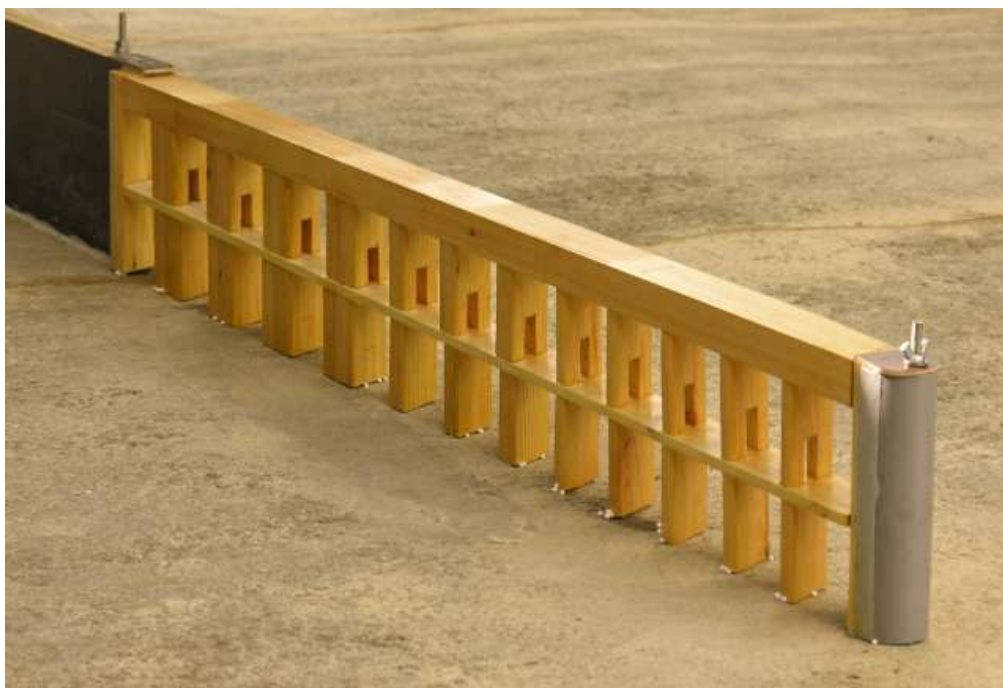
Figure 11: Layout C, downstream: final layout of the openings, seen on the scale model.
