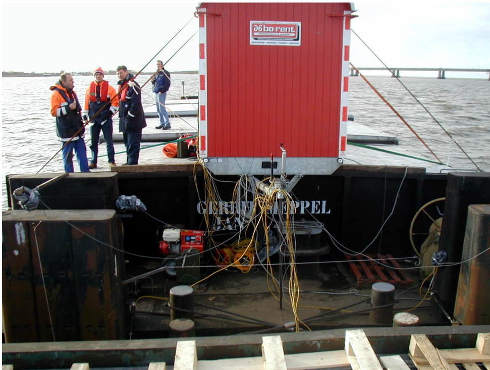
Photograph of the pushtow sailing to open water to carry out prototype measurements for the SHIP-MOORINGS validation of pushtow simulation model.
