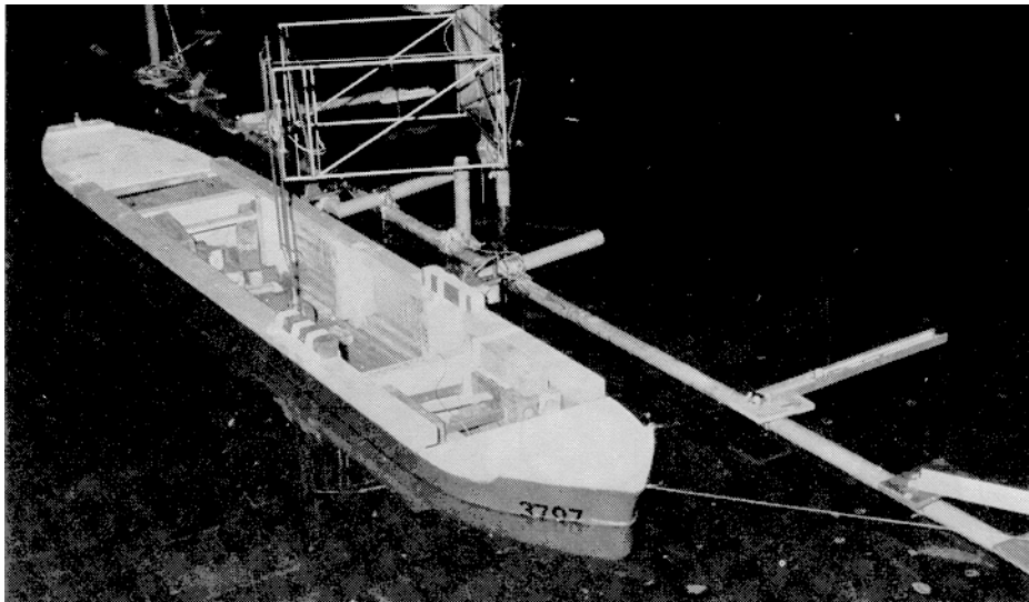
Figure 3.2 Experimental layout of moored ship
